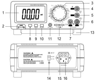
1. LCD 2. Power switch 3. Function knob 4. V $\Omega$ Hz input terminal 5. COM 6. Less than 2A 7. 20A current input terminal current input terminal 8. Backlight switch 9. Hold switch 10. AC+DC measuring switch 12. Capacitance measuring plug 14. 110V/220V 11. hFE plug 13. Bracket transfer switch 15. Fuse 16. Power plug
